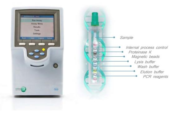
and deliver real-time PCR results less than 30 minutes\*.
